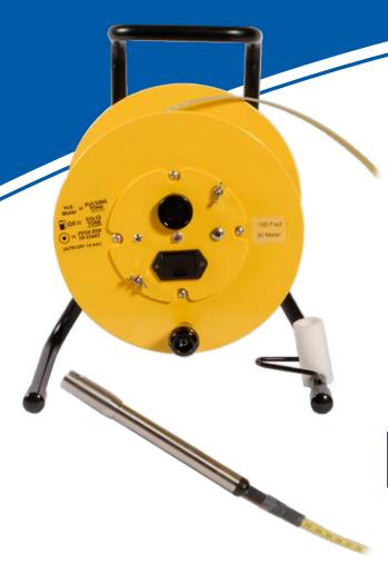
Combined system to accurately measure water level and detect hydrocarbons in potentially contaminated wells.
